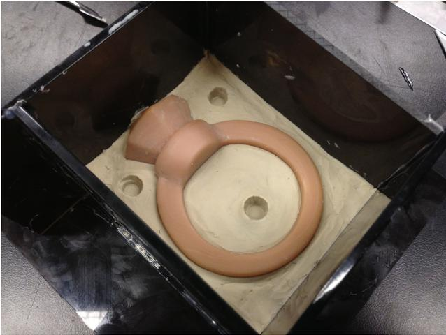
**Figure 7.** Registration keys pressed into the surface of the clay.
