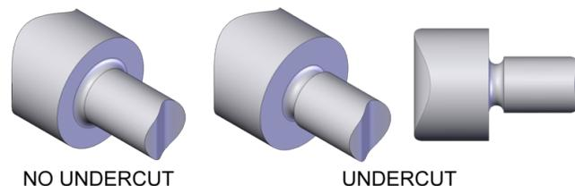
**Figure 1.** An example of an undercut in a part.
