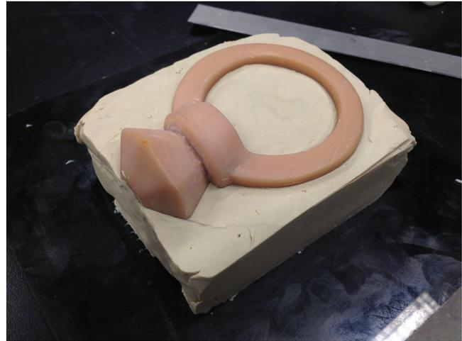
**Figure 6.** Oil clay built up to the parting line.
