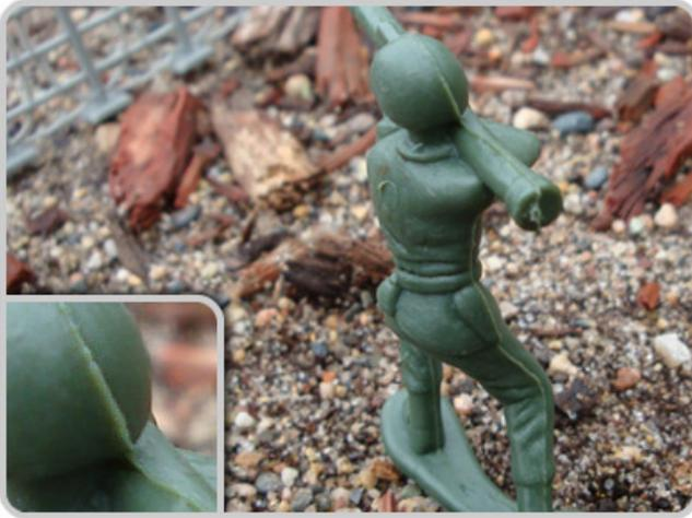
**Figure 2.** Excess material indicates the location of the parting line.
