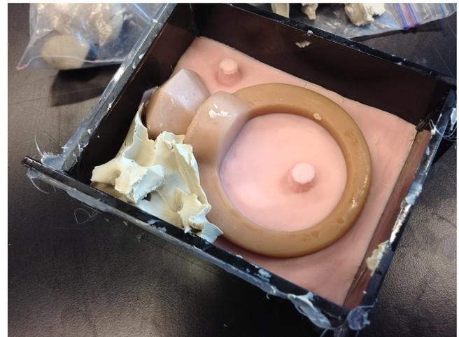
**Figure 8.** Peeling back the clay to reveal the first pouring of silicone.
