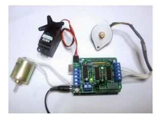
causing the teeth to move "one step" to orient itself with the charged electromagnet. An inner gear will then simultaneously move "one step," providing the motion that makes stepper motors so useful.
