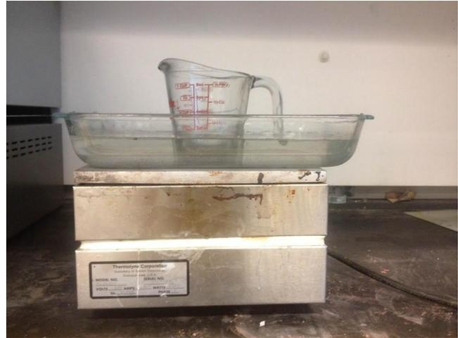
Figure 4. Hot plate double boiler setup.
