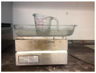
Figure 4. Hot plate double boiler setup.
